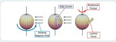
• The spherical fly wheel can rotate in a three dimensional direction, and a torque in a three-axis direction is generated.
